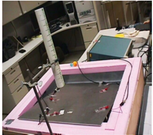
FIG. 3. (Color online) Photograph of the ball drop experimental setup. Vertical pipe above the inclined plate guides the ball drop path.
