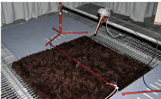
FIG. 2. (Color online) Experimental setup for the measurement of normal acoustic impedance at oblique incidence using a spherical sound source. The synthetic hair material is shown with a random fiber alignment.
