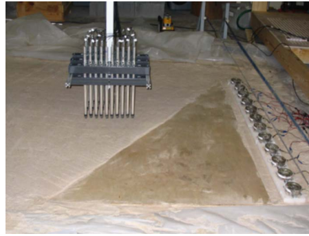
Fig. 1. (Color online) The experimental facility. The seismic transducer array is on the right and the ground-contacting sensor array is positioned over the sand tank. The plywood wedge-shaped asymmetric surface layer is buried flush with the surface of the sand.
