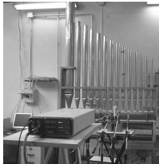
FIG. 1. A sketch of the setup indicating the position of the laser and the microphones; p1, p2, and p3 correspond to the selected measurement points.
